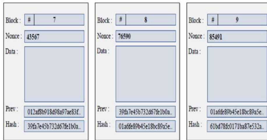
Figure. 1 Structure of bitcoin blockchain for three the blocks (Bhabendu 2019)
