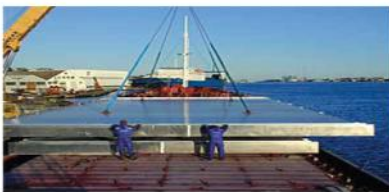
Figure –3 Marine Aluminium preferred FSW desk panels for the world cruise ship
