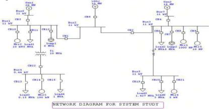
Fig 1: Single line diagram of the study
