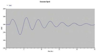
Fig 14: Generator speed for transient study case area 1
