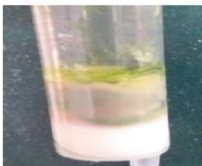
Figure 5. Expression of the colour bands of photosynthetic pigments by silica gel column chromatography in the DPJ of green and red spinach leaves.
