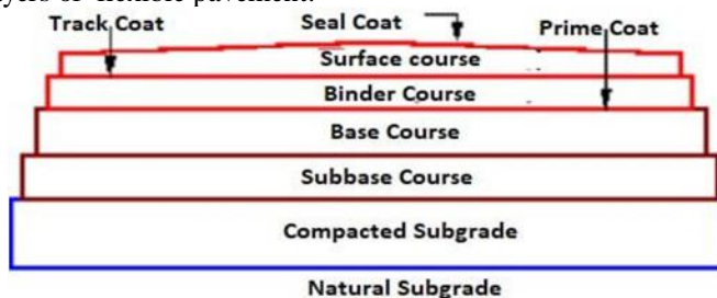
Fig0.1: Typical layers of flexible pavement
